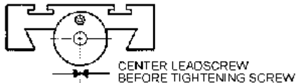
FIGURE 2--Make sure the lead screw is centered. Using the handwheel to run the table all the way in (away from the operator) before changing thrust collars will make this easier to do.
