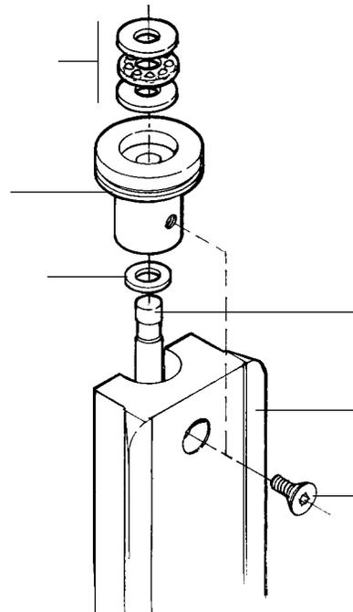
when the screws are tightened, you can remove the housing shell and sand the mating surfaces on a piece of sandpaper on a flat surface until they grip the collar tightly enough.
