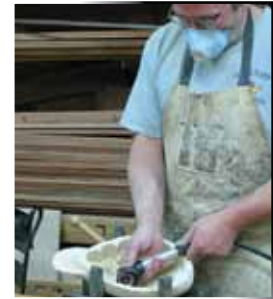
Carpenter and woodcarver, Ted Knapp, uses a Typhoon Disc to hollow out a decoy.
