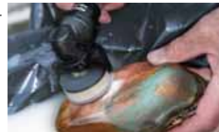
Using AR10046 Sanding Head with PSA Flex Diamond psa disc on California Jade.
